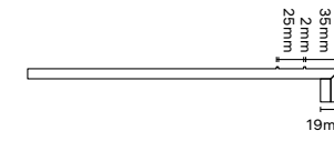
step tread "L" corner inox . nez de marche "L" angle inox ecke stufenplatte "L" inox . degrau "L" canto inox
